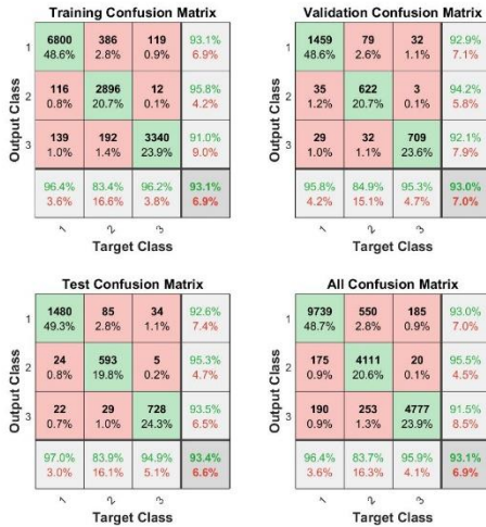
Figure 12 - Confusion matrices of all steps in a learning process of an ANN, in this specific case 20000 normalized entries with noise added
