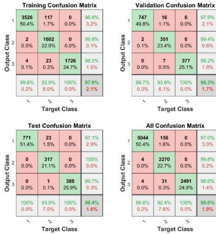
Figure 11 - Confusion matrices of all steps in a learning process of an ANN, in this specific case 10000 normalized entries with no noise added
