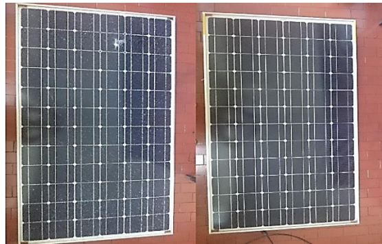
Figure 2 - The two panels tested in the laboratory: left side (broken glass and a broken cell), right side (healthy panel)
